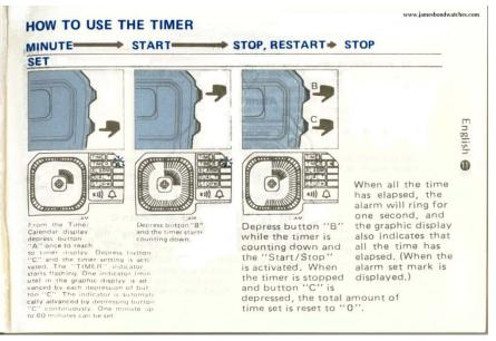
^ From the Time/Calendar display depress button "A" once to reach to time display. Depress button "C" and the time setting is activated. The "TIMER" indicator starts flashing. One indicator (minute) in the graphic display is advanced by each depression of button "C". The indicator is automatically advanced by depressing button "C" continuously. One minute up to 60 minutes can be set.
